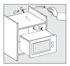
Push the microwave oven into the niche and pull the cable with the plug through the back of the unit.
